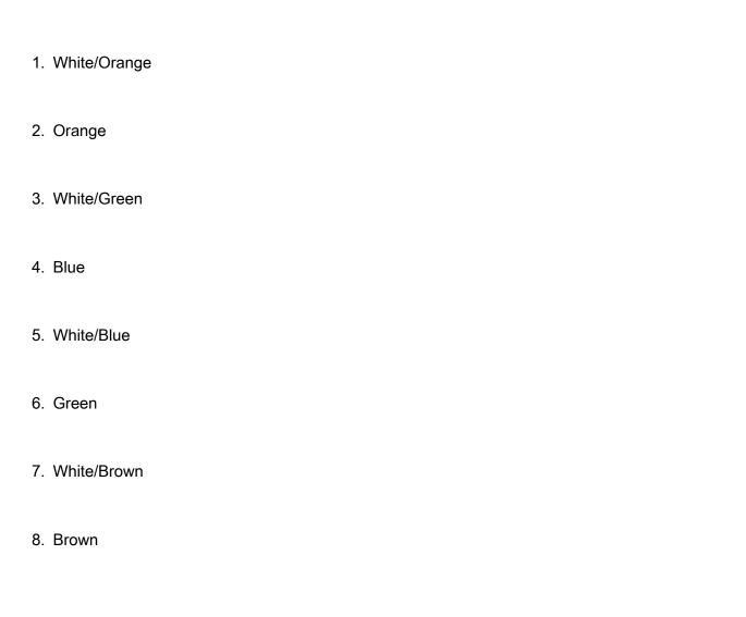
T568B is the most commonly used wiring scheme in commercial installations across the United States and is widely accepted in modern networking environments.
